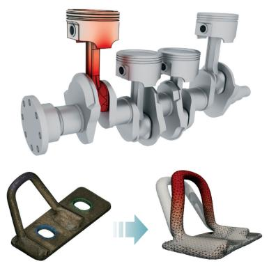
Coreform IGA can run simulations directly on STL surface meshes.
