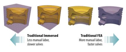
**Illustration above** — Coreform's "Flex IGA" technology, where CAD geometry can be progressively fit more tightly with the spline simulation domain to enable faster solve times.
